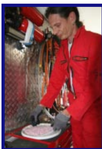
A job just for a shot firer SECUTAG® is being admixed to the explosive.
